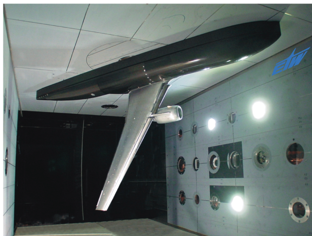
Fig. 2 KH3Y stage 3 high-lift configuration model in ETW.
